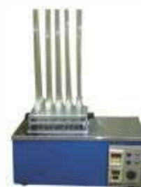
COD DIGESTION UNIT
